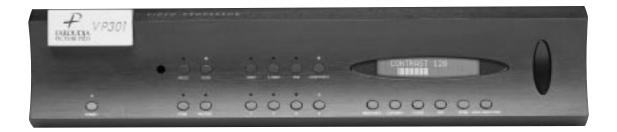
The Faroudja VP301 Line Multiplier is a precision video instrument used to convert NTSC interlaced signals into 600 visible, progressively scanned lines (800X600 resolution). Using Picture Plus<sup>™</sup> technology, the VP301 removes typical video processing artifacts while also increasing color purity and image detail, closely matching 35mm film.
