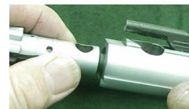
“GENTLY” insert bolt in carrier. You may need to compress the outer ring with your fingers to ease initial insertion. **DO NOT FORCE!**
