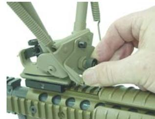
3. Tighten Bipod Pivot Tension.
