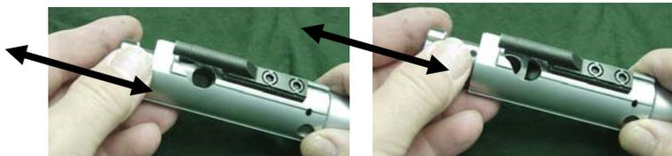
If bolt slides in and out of bolt carrier too easily, the 2-piece bolt ring set needs to be replaced. Worn out rings can lose gas and cause malfunctions like “short stroking” because the bolt carrier is not propelled far enough rearwards during recoil.
