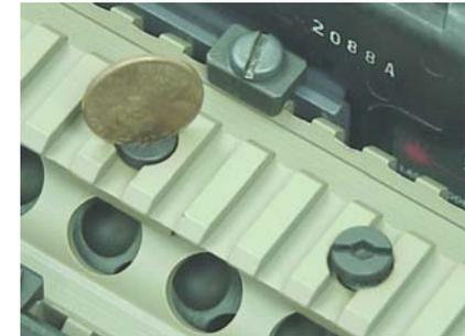
Note: Newer Screws are also slotted for turning with a coin.
