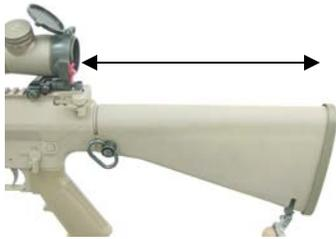
Move scope forward for eye relief with stock at shortest position.
