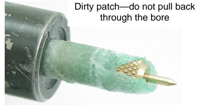
*Once patches wet with bore cleaner clear the muzzle and are reasonably clean, then scrub the bore with the brass bore brush. After 5 full in-and-out strokes with the bore brush, change back to wet bore patches as described previously.*
