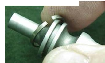
1. Inner ring install starting position. Using your fingers of the supporting hand, keep the top end ring as much in the groove as possible...
