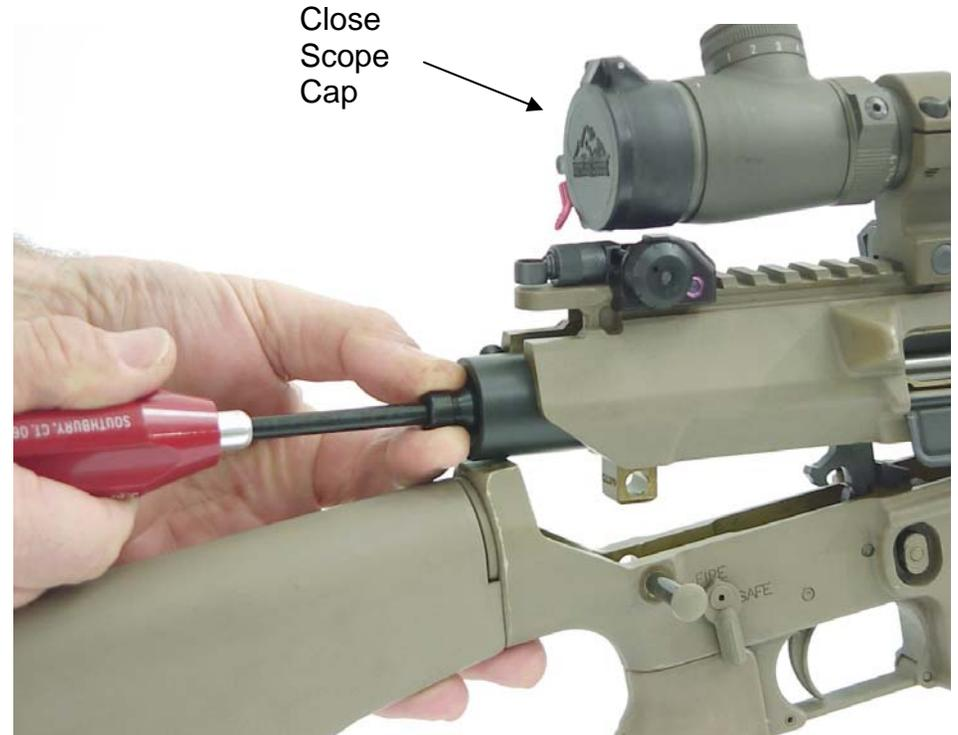
**Note:** If your cleaning patches are too large they may be too difficult to push through the bore, either cut down the patch to reduce its size, or remove the bore rod tip or jag from the rod and try just the rod end to push patches through.
