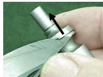
A pen knife is a field expedient tool to remove the old rings. Pry up one end and push ring rearwards of bolt.
