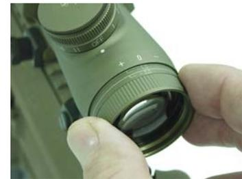
(3) Once at the best focus point, turn the eyepiece back and forth through the focus point until the reticle is at its maximum sharpness.
