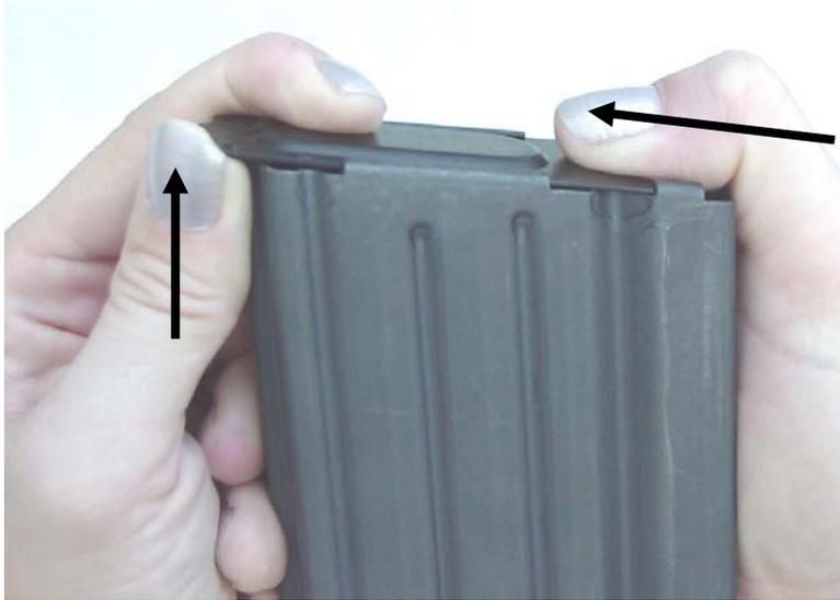
Figure 2-5b Removing Magazine Base
