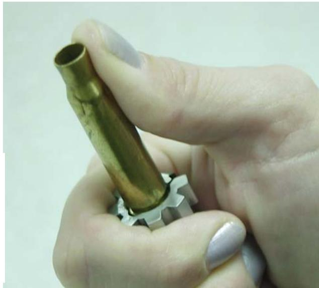
FIGURE 3-1 Ejector Cleaning Procedures
