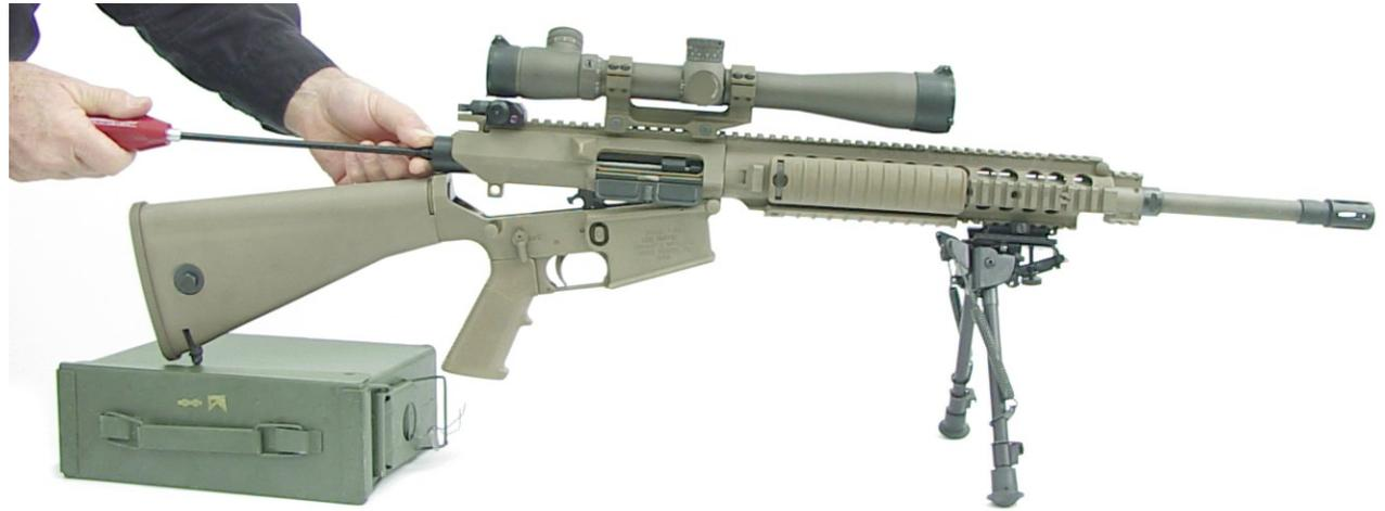
*Using the Bore Rod Guide in this manner helps keep the sights up, and if the buttstock is raised as shown above, then bore solvent drains away from the chamber, while keeping the rifle stable for bore cleaning.*
