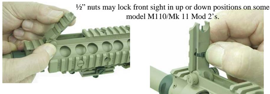
Figure 2-6d Deploying M-110 Front Sight
