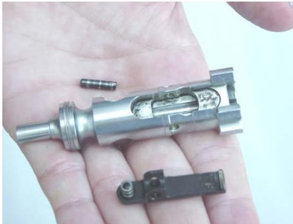
Bolt & Extractor readied for detail cleaning.
