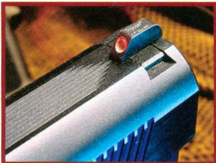
Front sight is a ramped blade from STI housing a tritium dot. Note serrations on the flat-top slide.
